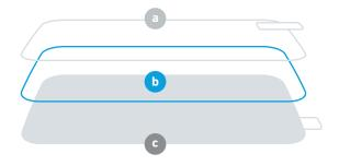
Cap Sheet Clear, rigid sheet covering the protective film.
