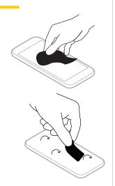
4 Remove new protector from plastic backing. Line up protector at one end of screen and lay onto phone.
