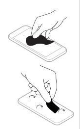
4 Remove new protector from plastic backing. Line up protector at one end of screen and use squeegee to lay onto phone.
